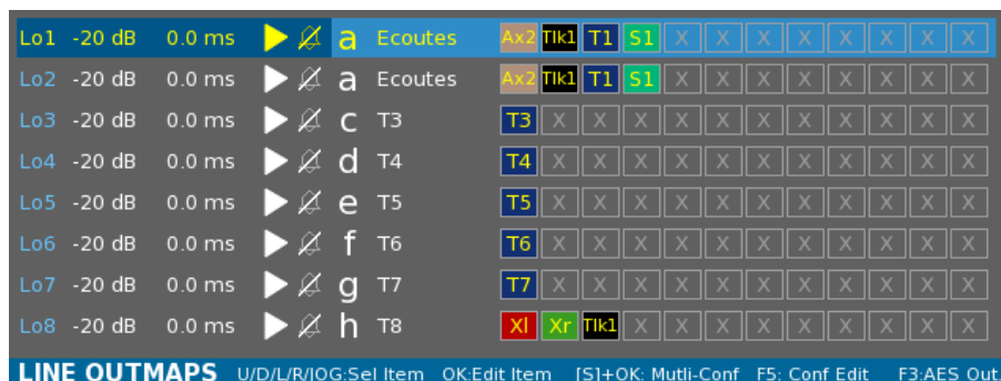
The management of SubGroups and Auxes on the Line Outmaps page: here, the Aux 2 "Ax2" and SubGroup1 "S1" have been assigned to Listening Configuration A, renamed "Ecoutes", and sent to Line Outputs 1 and 2.
